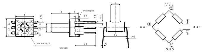
Output code because on into pressure port. 4 terminal is N/C, avoid to apply voltage.
