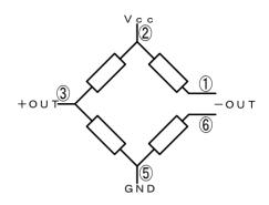
Output code because on into pressure port. 4 terminal is N/C, avoid to apply voltage.
